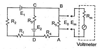
The voltage across AB is measured by a voltmeter whose internal resistance is  $9500 \,\Omega$ . What is the measurement error caused by the resistance of the measuring instrument?
