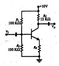
negative feedback by adding resistor  $R_{\rm E}$ . Find the value of resistor  $R_{\rm E}$  using
